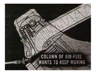
In a naturally aspirated engine, on the intake stroke, the piston drops creating an area of low pressure in the combustion chamber that is less than atmospheric pressure and as the intake valve opens, the air from the outside is set in motion down the IM runner.
