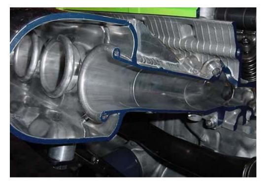
Jun IM Cutaway showing the velocity stack opening for the runner inside the plenum.
