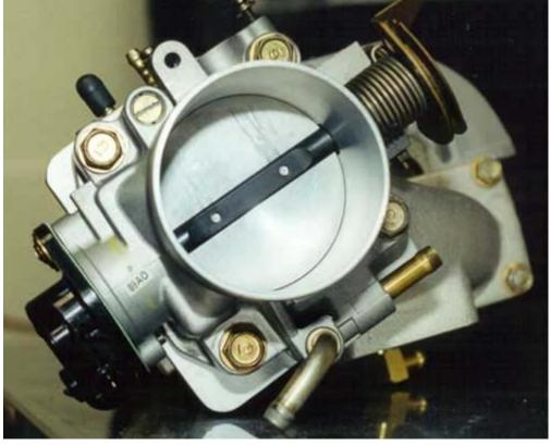
Once we have determined the optimal TB size for our IM, we can then determine the best intake inner diameter.
