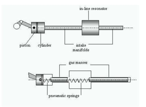
The analogy used by most mechanical engineers to explain how a resonance chamber works is that it acts like an oscillating spring (i.e. imagine the plenum acts like the spring) with a block attached on the end of the spring (imagine the air wave in the IM runner to behave like the block). As the block compresses the spring, the spring builds or stores up energy and when the spring uncoils, the block is given a push or energy as it travels away from the spring's compressed position.
